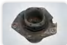
Torn Strut Insulator
